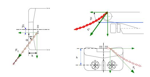
Figure 2.7.2 – Diagrams showing the intended meaning of parameters  $\alpha$ ,  $\beta$ , x, y and h.  $F_t$  shows the vector of the applied wire tension."
