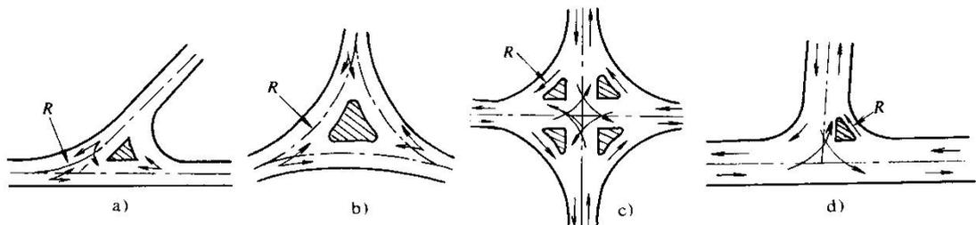
Fig. 10.3 Channelization (placing turning lanes)
