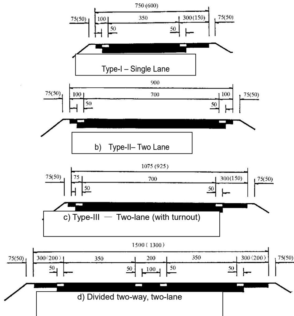
**Fig. 11.3.2 Basic Ramp roadway Cross-sections**
