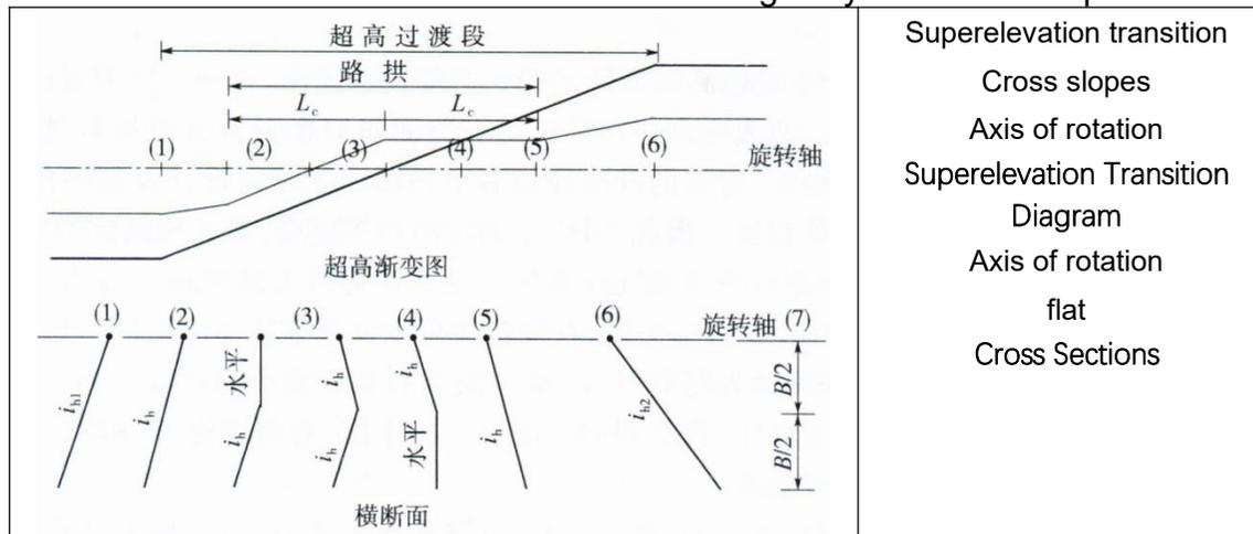
Fig. 7.1 Superelevation with additional crown lines
