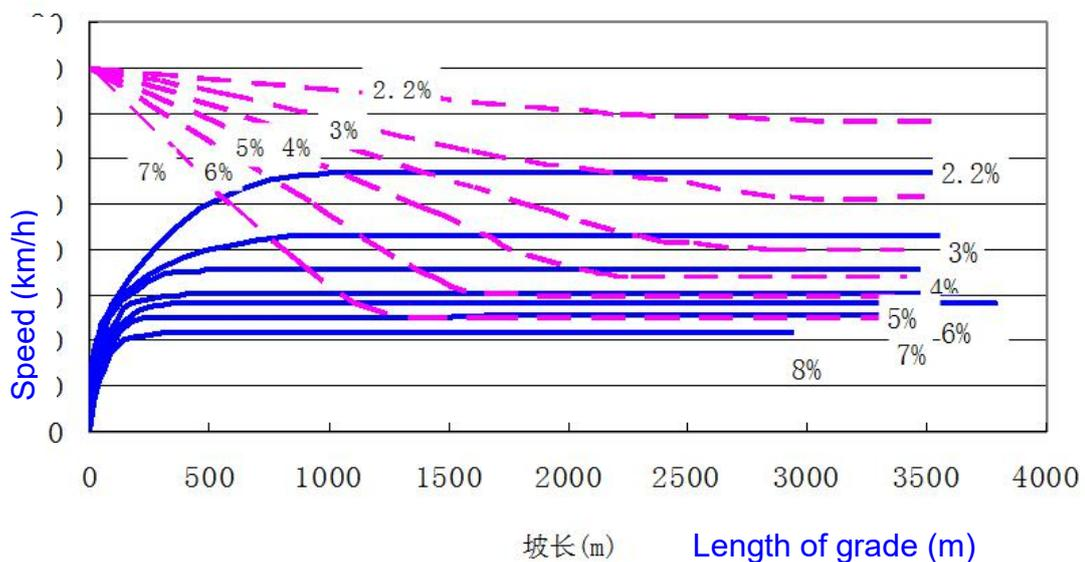
Figure 8.1 Upgrade Acceleration and Deceleration Curves of Two-Axle Loaded Trucks (12.6t and 14.15t, power/mass ratio of 9.3kw/t)
