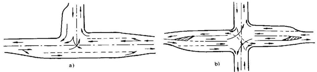
Fig. 10.2 Channelization (widening of approaching legs and placing turning lanes)
