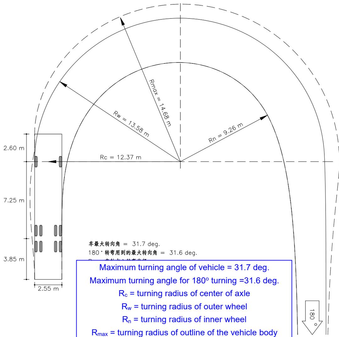
Fig. 10-7 Minimum Turning Radius of Large Bus (m)
