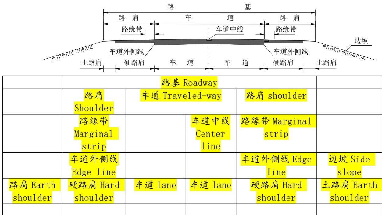
Figure 6.1.2-4 Typical cross-section of class-2, class-3 and class-4 highways
