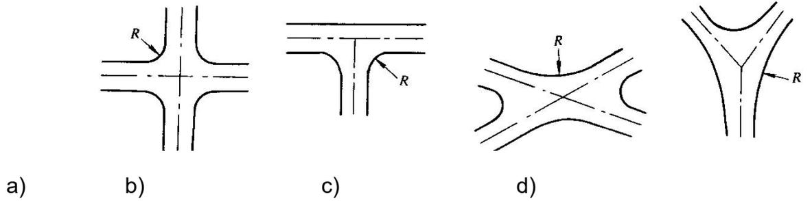
Fig.10.1 Channelization (widening turning corners)
