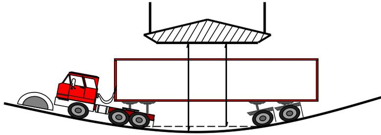
**Figure 6.6.4 Effective vertical clearance on a sag curve**
