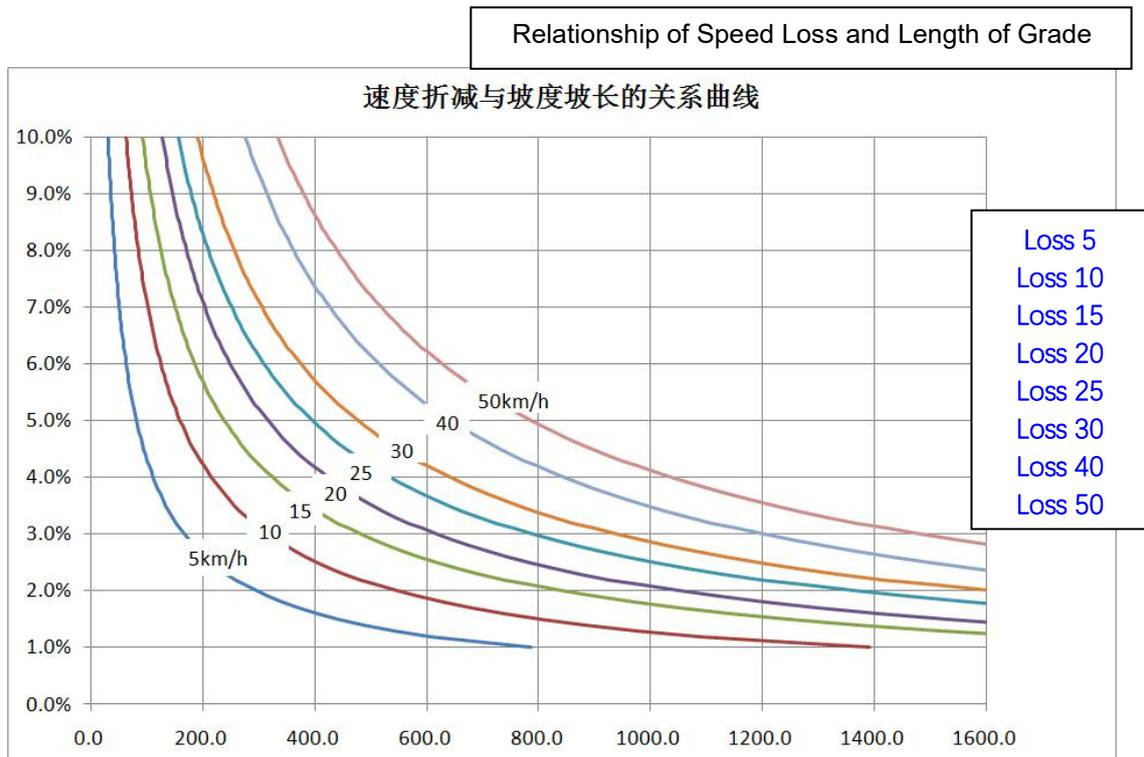
Fig. 8.4 Speed Loss of Fully Loaded (49t) 6-Axle Articulated Trailers
