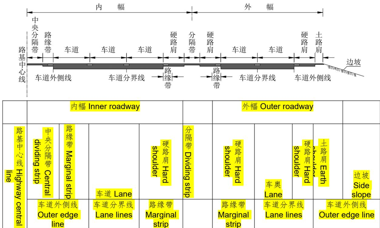
Figure 6.1.2-3-2 Integral Type combined cross section (right roadway only) of a motorway
