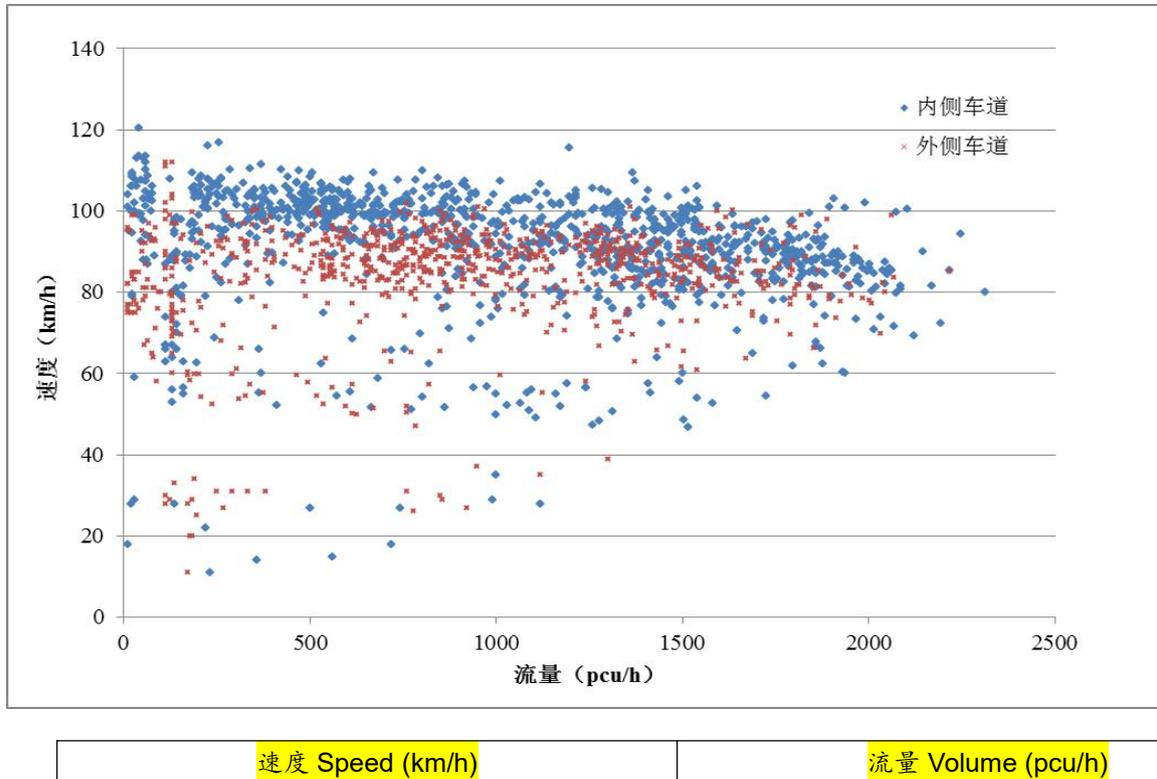
Fig. 3.1 Motorway speed-volume relationship
