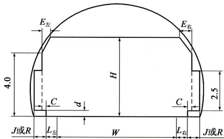
Figure 6.6.2 Clearance profiles of classified highways ( unit: m )
