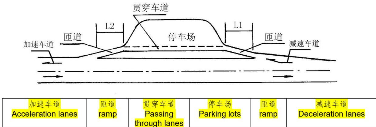
**Fig. 13.3.3 Layout of a service or rest area**
