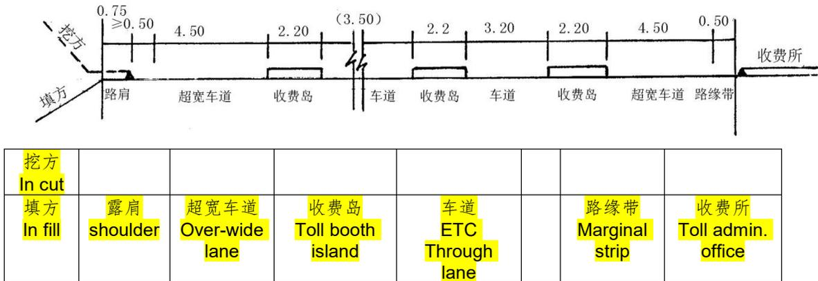
Fig.13.2.2-2 Roadway Cross-section at Centerline of toll plaza
