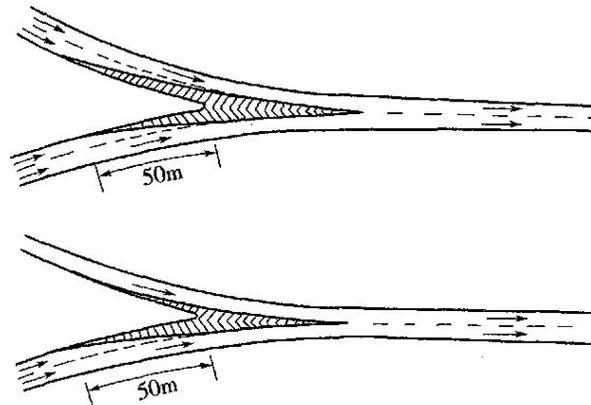
**Fig 11.5.4 Lane Reduction before Merging**
