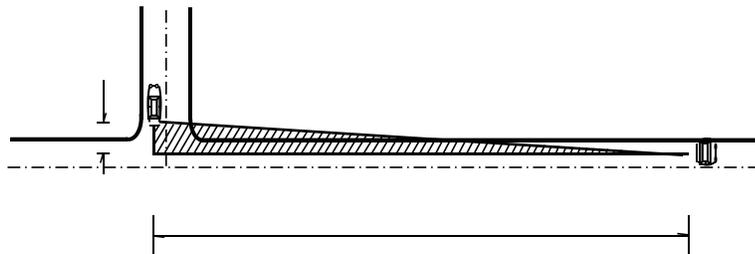
**Fig. 10.3.2-2 Sight Triangle of Stopping Sight distance for Safe Crossing**
