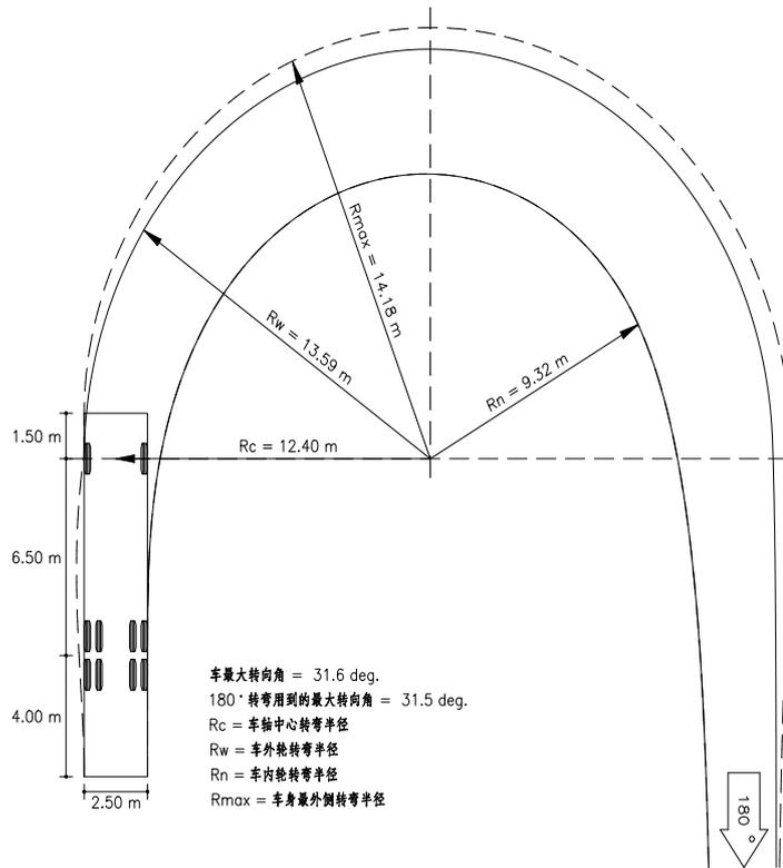
Maximum turning angle of vehicle = 31.6 deg.
