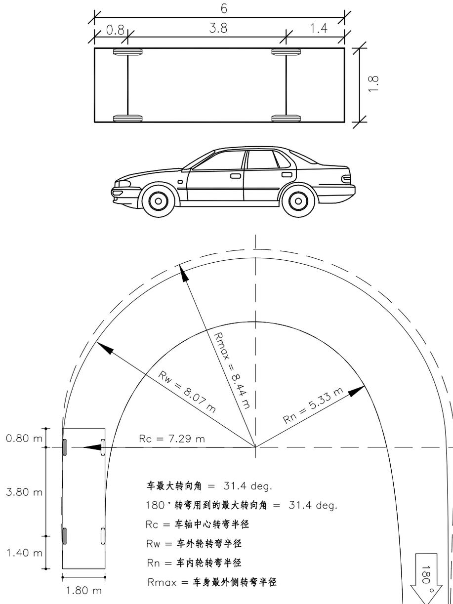
Maximum turning angle of vehicle = 31.4 deg.
