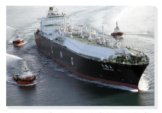
A membrane-type LNG carrier with a capacity of 147,000 cu m built by China
