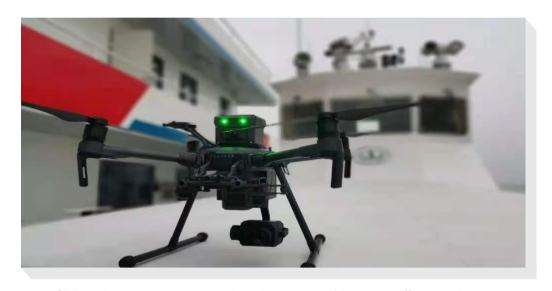
Ship exhausts remote sensing drone and airborne sniffing equipment
